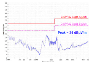
Figure 12. Radiated EMI Result from the Two Layer Board
