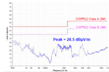
Figure 13. Radiated EMI Result from the Four Layer Board with Unbroken Ground Planes
