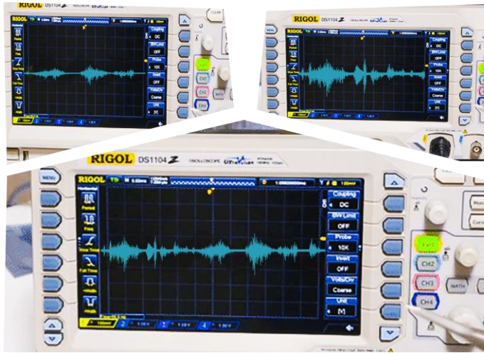
Figure shows failed measure signal where Noise occurred at output data.
